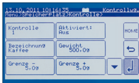
40 memories for each mode , for checkweighing, pre-tare, reference weight, target weight when dispensing etc.
